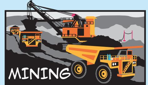
MINING IS USED WHEN OIL SANDS ARE CLOSE ENOUGH TO THE SURFACE TO BE DUG UP USING EXCAVATORS, WHICH LOAD IT ONTO LARGE TRUCKS. THE **OIL SANDS** ARE TAKEN TO A PROCESSING PLANT WHERE IT IS MIXED WITH HOT WATER TO REMOVE THE SAND AND CLAY.
