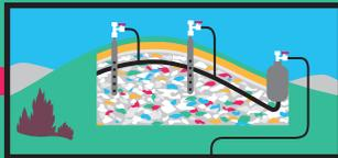
**LANDFILL GAS CAPTURE:** METHANE FROM CAPPED LANDFILLS IS COLLECTED, PROCESSED AND UPGRADED, THEN TRANSMITTED BY PIPELINE TO HOMES AND BUSINESSES.
