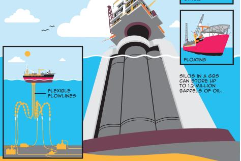
IN A FPSO VESSEL SYSTEM, FLEXIBLE FLOWLINES ATTACH TO WELLHEADS IN THE SEAFLOOR, WHICH ALLOWS FOR THE VESSEL TO MOVE AROUND TO ADAPT TO WEATHER CONDITIONS. THE EXTRACTED OIL IS THEN SHIPPED TO SHORE BY SHUTTLE TANKERS.
