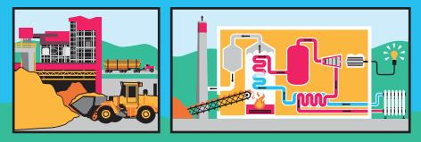
ELECTRICITY: WOODCHIPS, SAWDUST OR OTHER ORGANIC MATERIALS ARE COLLECTED AND COMPRESSED INTO PELLETS. THE PELLETS FUEL A BOILER USED TO PRODUCE STEAM. IT TURNS TURBINES, WHICH SPIN MAGNETS IN A GENERATOR, CONVERTING MECHANICAL ENERGY INTO ELECTRICITY.
