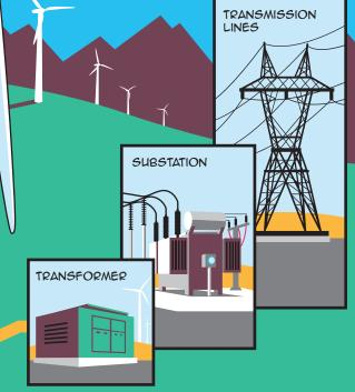
A TRANSFORMER INCREASES THE ELECTRICITY TO A HIGHER VOLTAGE, TRANSMITTING IT TO A SUBSTATION THAT INCREASES THE VOLTAGE AGAIN SO THAT IT CAN TRAVEL OVER LONGER DISTANCES THROUGH THE ELECTRICITY GRID.
